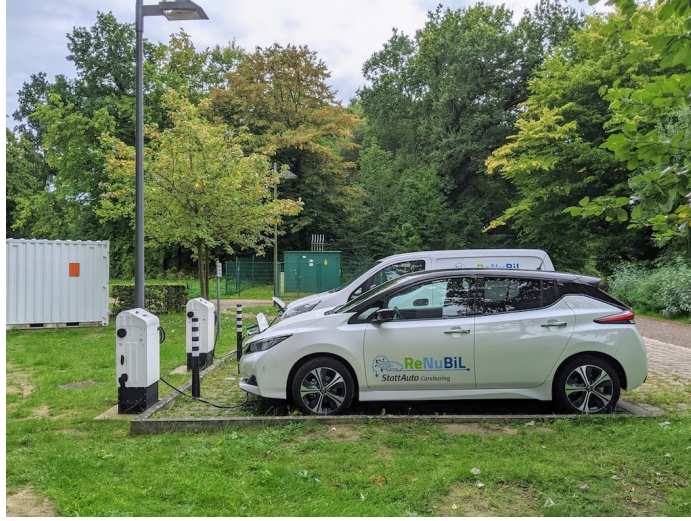
Fig. 1. ReNuBiL living lab on University of Lübeck’s campus with two electric cars, two bi-directional charging stations, and stationary battery container
